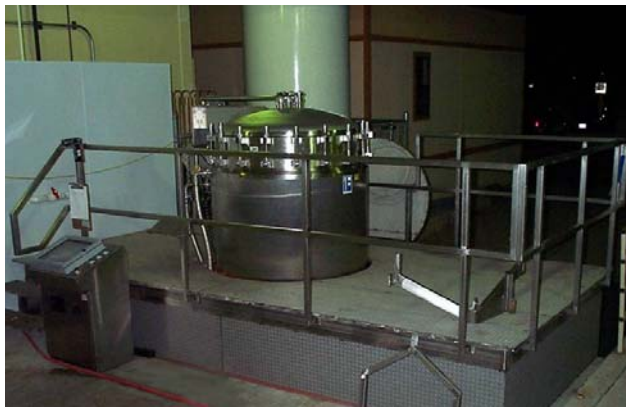
FIGURE 1. Example alkaline hydrolysis tissue digester with 2,000 lb capacity (Powers, 2003).
